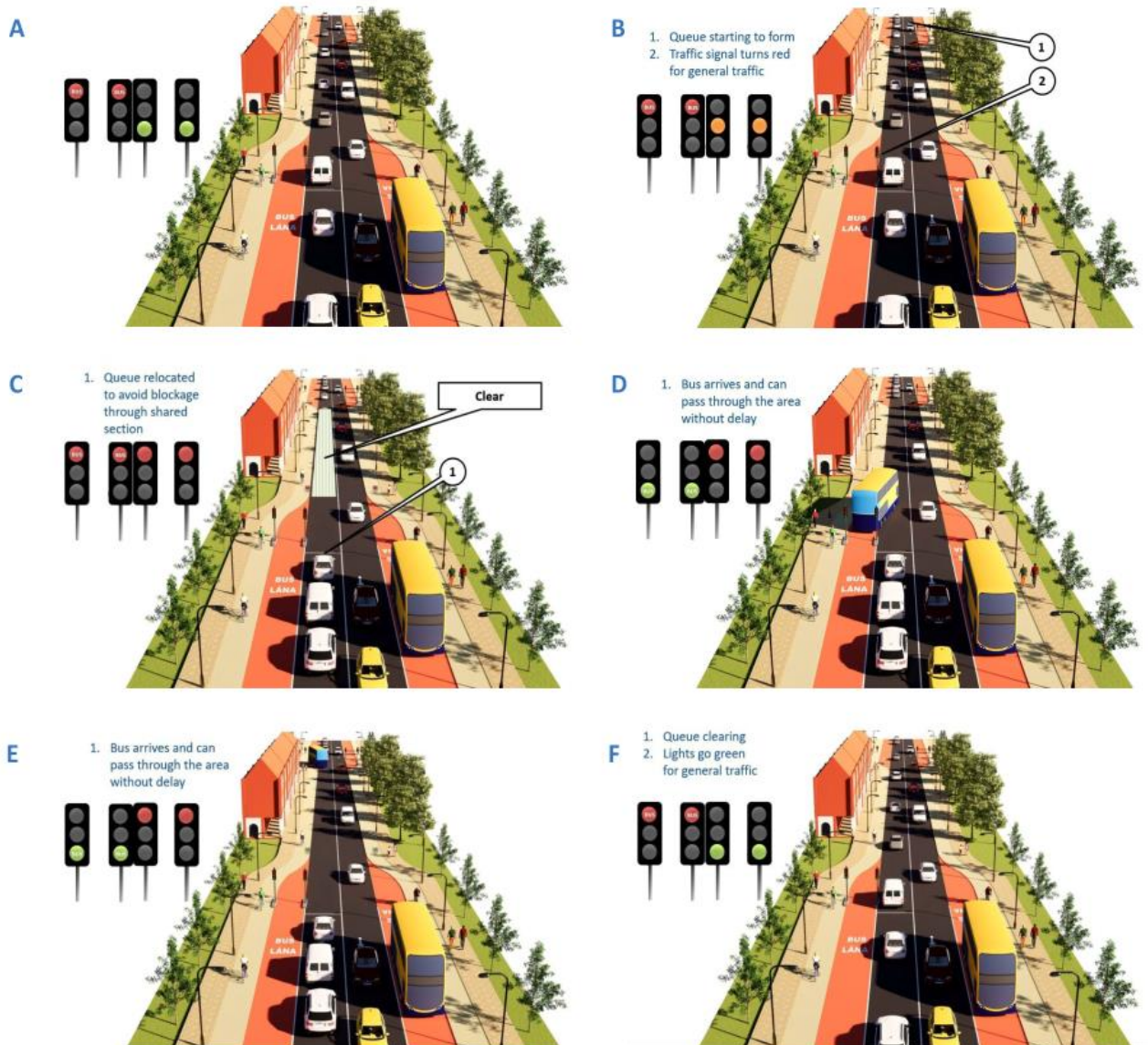
Image 4.7: Signal Controlled Priority Schematic Operation (Source: PDGB)
